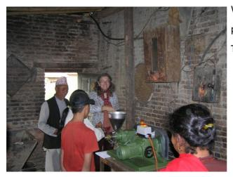
We could finally install a screw press for the production of high value seabuckthorn seed oil. The press can be also used for other oilseeds.
